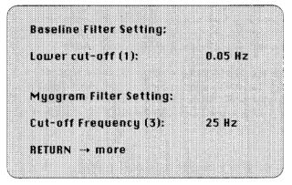
The digital **baseline filter** has been designed in order to suppress excessive baseline drifts. By pressing key 1, the setting can be altered to one of the following values: 0.50, 0.25, 0.12, or 0.05 Hz. The value set is the lower limit of the frequency range and is normally set to 0.05 Hz, ie a frequency range of 0.05 to 100 Hz.
