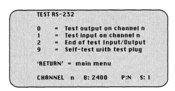
To test the RS-232, connect the CARDIOVIT AT-3 to an external unit.
