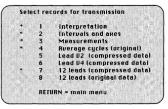
By pressing the indicated characters (1 to 8), the data to be transferred can be freely combined. The choice is indicated by an asterisk (\*).
