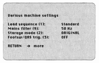
The **lead sequence** can be switched from Standard to Cabrera and vice versa by pressing key **1**.
