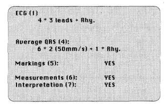
In the ECG section, the format of the printed leads can be selected. By pressing key 1, different format possibilities appear on the screen.
